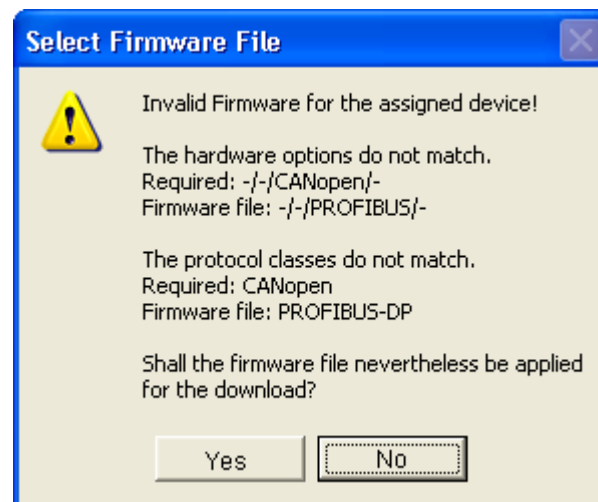
Figure 19: Request Select Firmware File - Example Invalid Firmware
